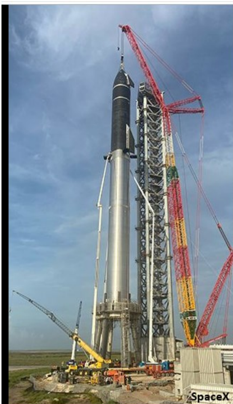
The American SpaceX company has made the biggest rocket ever constructed. The vehicle has two segments - an upper-stage called Starship and a booster called Super Heavy. There are 29 methane-burning engines at the base of the Super Heavy booster.
