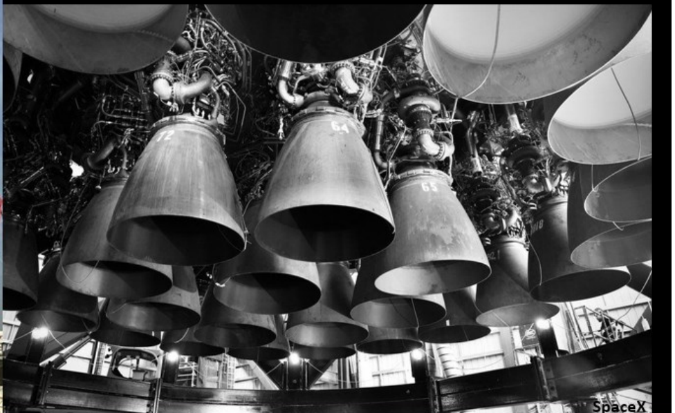
The American SpaceX company has made the biggest rocket ever constructed. The vehicle has two segments - an upper-stage called Starship and a booster called Super Heavy. There are 29 methane-burning engines at the base of the Super Heavy booster.
